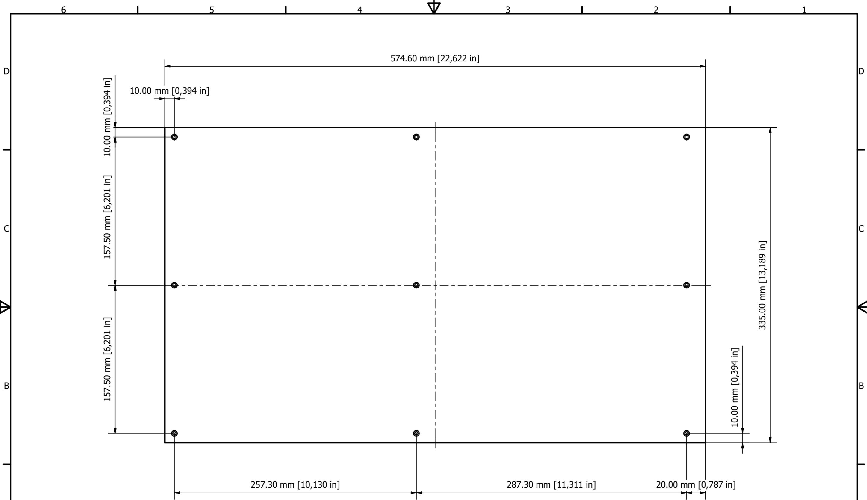
Mounting plate is made from 1.5 mm unfinished aluminium.
