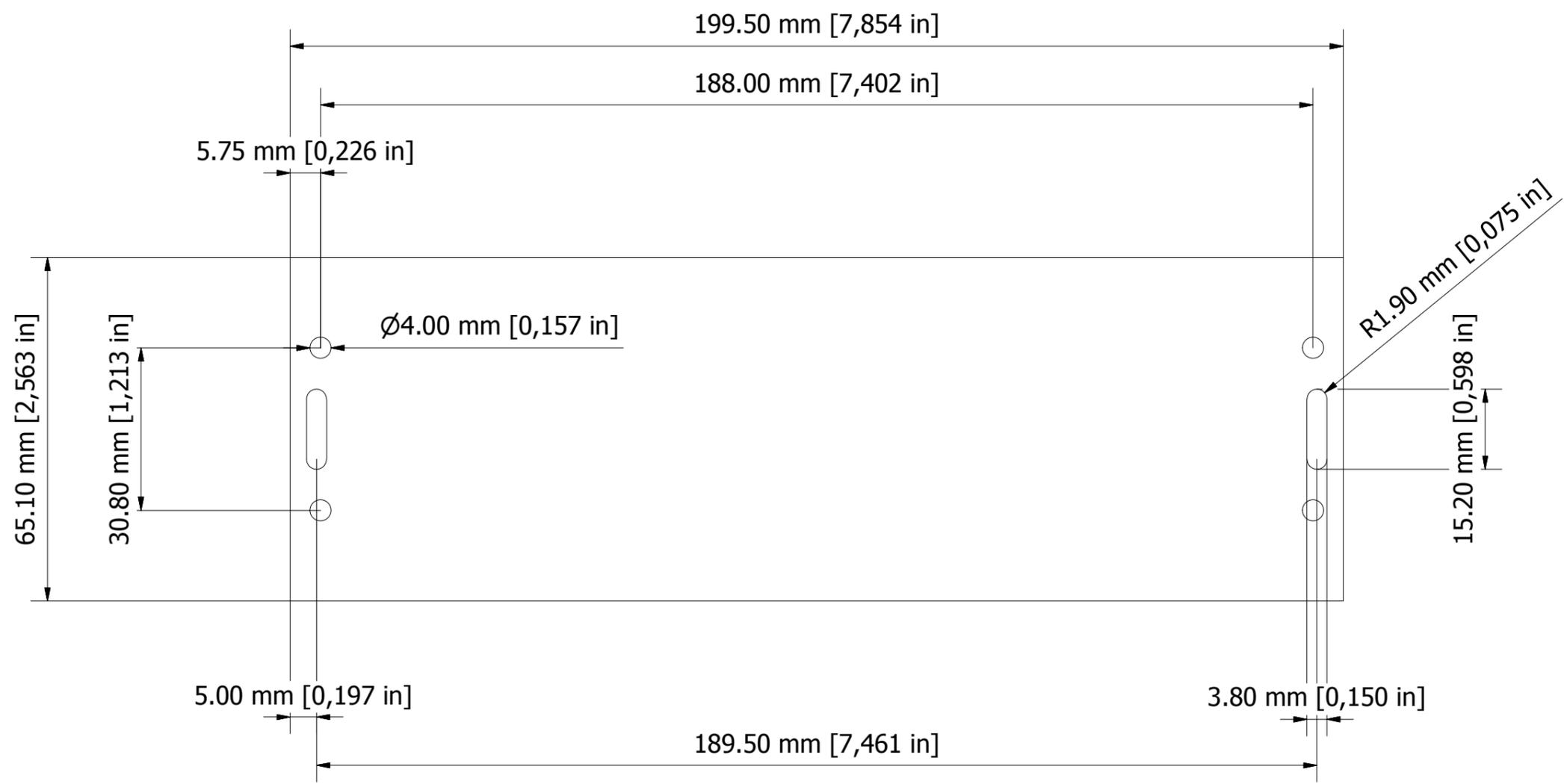
Material is 2mm aluminium with an etch and clear anodise finish.
